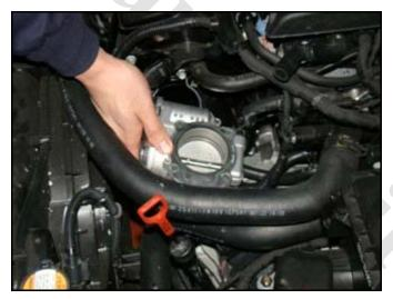
4. Spray a carbon cleaner or throttle body cleaning solution on the throttle valve and bore areas where deposits have accumulated. Wipe off the deposits with a clean and soft shop towel (as shown in the pictures).
