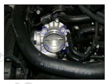
**NOTE:** Do not disconnect the coolant hose from the ETC throttle body. It is not necessary to remove the ETC throttle body completely from the vehicle for cleaning.
